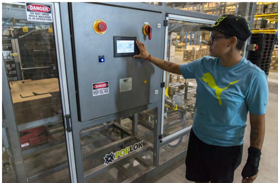
Built with a heavy-duty welded steel frame, the rugged PopLok tray-forming machine is controlled via an Omron PLC (programmable logic controller) and features an operator-friendly HMI (human-machine interface) for easy navigation.
