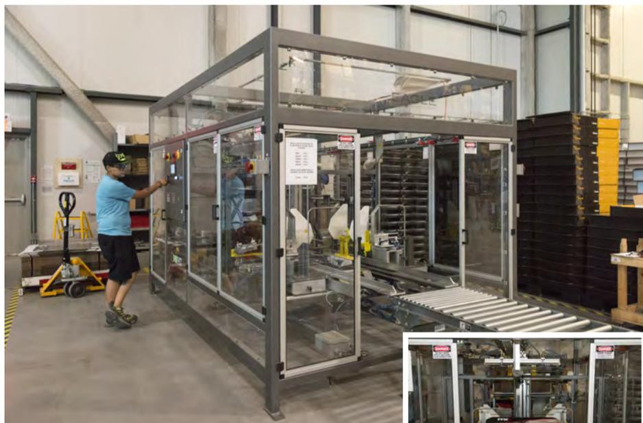
The fully-automatic PopLok tray-forming solution is a turnkey workcell currently used to make 12 packaging-ready corrugated retail boxes per minute for the facility's picking tables handling control arm products.
